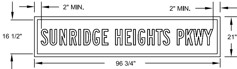
STD. 12" EXTRUSION WITH 1-1/2" TOP HINGE RETAINER SYSTEM
