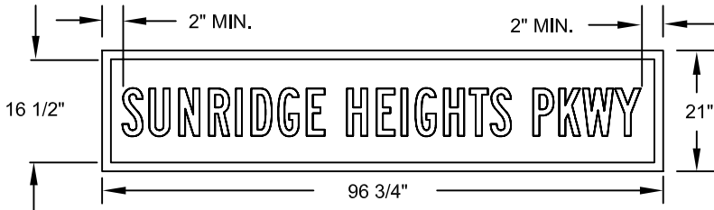
STD. 12" EXTRUSION WITH 1-1/2" TOP HINGE RETAINER SYSTEM
