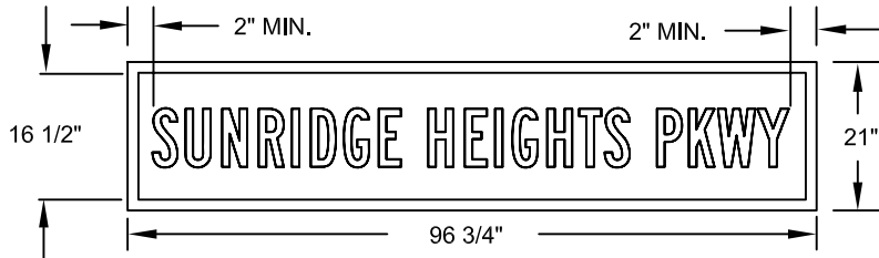
STD. 12" EXTRUSION WITH 1-1/2" TOP HINGE RETAINER SYSTEM
